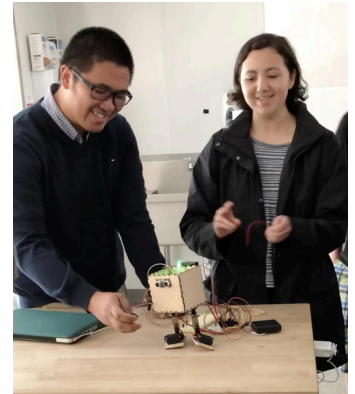
Berkeley undergraduates Jeffrey N. and Chelsey C. use servomotors and a distance sensor to make an environment-aware walking robot.
